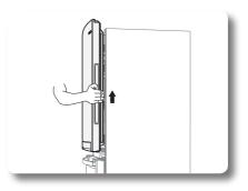
6. Remove the fridge door by lifting it upward. Be careful not to drop and scratch the fridge door.
